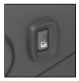
You can lock or unlock all doors on your vehicle from the driver's or front passenger's door lock switch.
